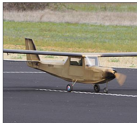
The biggest model flown was this modified Bud Nosen Trainer built by Paul Starks. Spanning 102", it featured electric power and a unique gold and black rattle can paint finish. Plane was a gentle giant in the air. Cogdell pic.
