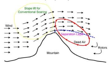
While flying this tilted circular path on the back of the slope, the glider crosses the boundary layer (separation layer in the figure) into the lift for a portion of this path.
