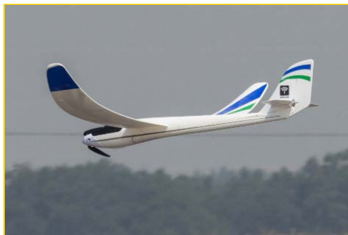
To reduce drag, the prop folds back when motor stops.
