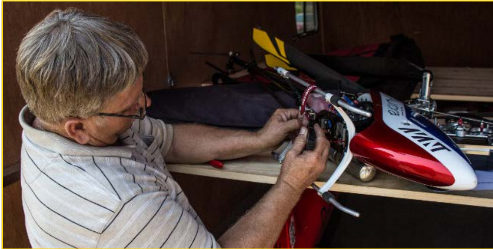
Don Coleman prepping a chopper to be flown by Don and his son, Steve. The Aurora Avant is powered by an OS90 Hyper engine and has a 5' rotor arc.
