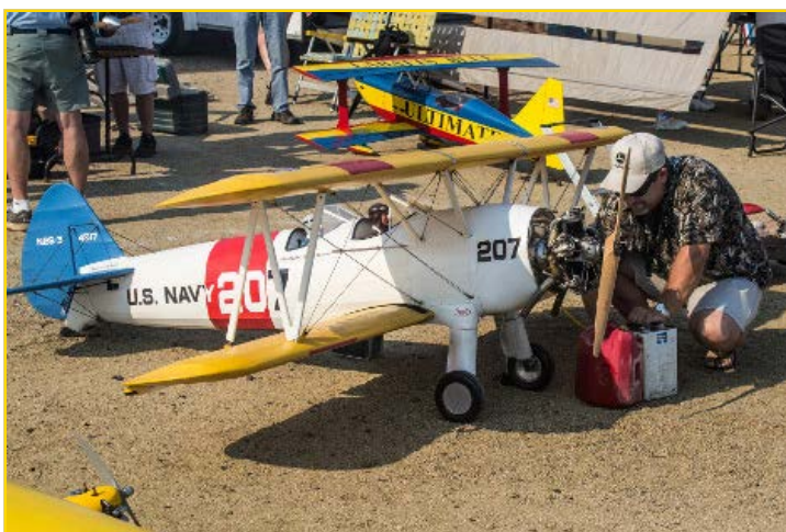
John Parks' 1/3 scale N2S Stearman was originally built by Martin Sherman and sports an RCS 215cc 5 cylinder radial that has to be heard to be believed. For more photos of this magnificent plane, see IMAA 2012 .
