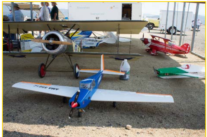
The plane with the blue fuse is Alan Littlewood's Mooney. It has a wingspan of 72" and is powered by an O.S. FS-61 four-stroke engine.
