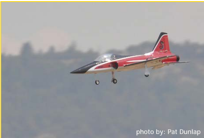
Doug McKee's all composite, 160mph, E-flite Habu 32 EDF ducted fan jet on approach.
