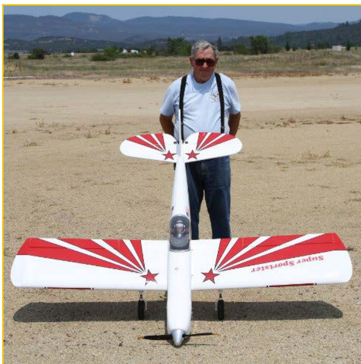
Martin Sherman with his 84 inch Super Sportster ARF, pulled by a Saito 36cc gas engine, and accentuated by classy Mustang wheels and struts. A little touch like the addition of these wheels and struts can turn a "ho-hum" model into a very classy bird.
