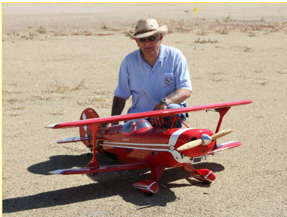
Martin Sherman with his 84 inch Super Sportster ARF, pulled by a Saito 36cc gas engine, and accentuated by classy Mustang wheels and struts. A little touch like the addition of these wheels and struts can turn a "ho-hum" model into a very classy bird.
