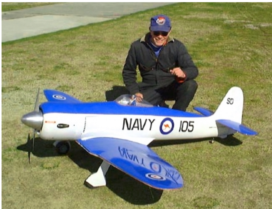
Fred Sargent shows his beautiful, 88 inch wing span Hawker Sea Fury. Fred made this plane from a kit by Dave's Custom Models. A 3W70cc 2-stroke engine turning a 20x12 prop powers it. Eleven servos move the usual control surfaces, plus several other moveable parts including flaps and landing gear. The model weights 31 to 32 pounds, and Fred says it flies very well. Fred covered the plane with cloth fiberglass and painted it very attractively.
