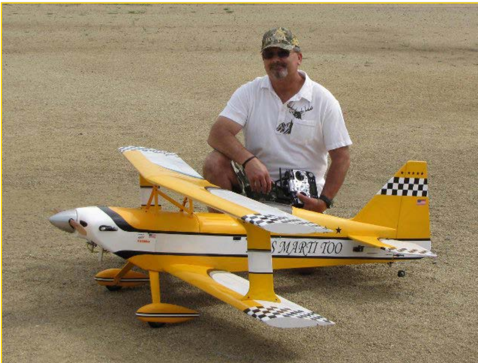
Jay Strickland and his Ultimate. This is another of those 'Take No Prisoners' Ultimates. This one has a wingspan of 72.5", weighs 21 pounds, is powered by an MT 70cc twin and has 32 flights. Jay flies this very deftly and makes it look easy... a sign of a very accomplished flyer.
