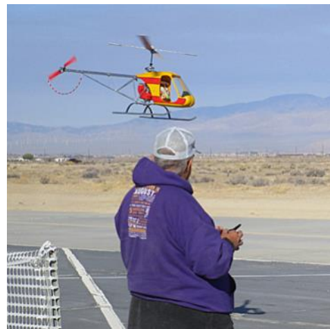
Tony Frackowiak flies his vintage Du-Bro Shark 60 that he fully restored. Early heli tech - glow power, no gyros.
