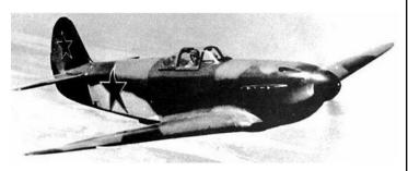
The Yak 3 was a highly maneuverable, low-altitude fighter-interceptor. All German pilots were taught to fear the Yakov-lev 3 because it could outturn, out-climb and out-accelerate both the Messeschmitt Bf 109 and Focke-Wulfe 190s at the low altitudes at which it tended to operate.
