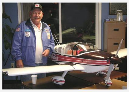
He built it from David Anderson plans, it weighs 35 pounds, power is a Zenoah GT-80, and finish is glass cloth with Klass Kote epoxy paint. John is planning to test fly in the Spring.
